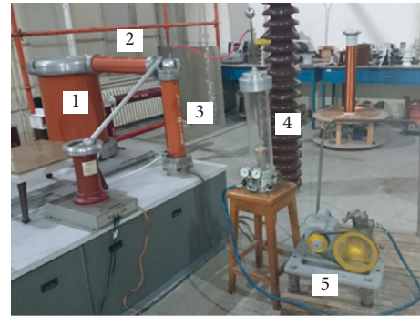
FIGURE 2: Test setup at high voltage laboratory of ITU. (1) Test transformer; (2) current limiting resistor; (3) capacitive divider; (4) test vessel; (5) vacuum pump.
